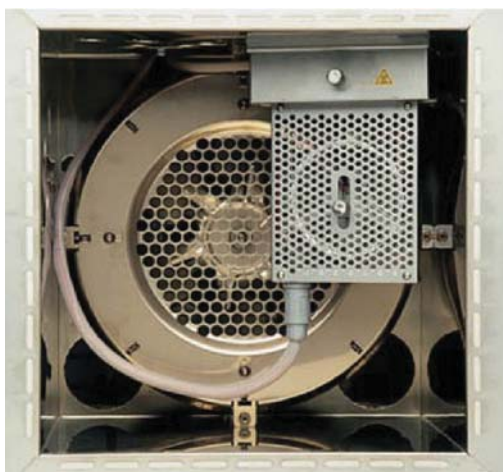
Figure 2.129 UFM column module installed in a regular GC oven (Mega, Legnano, Italy; TRACE GC Ultra, Thermo Fisher Scientific, Milan, Italy).
