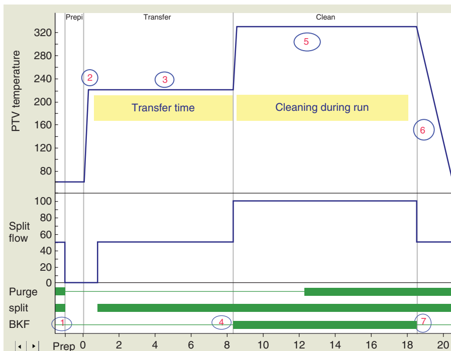
Figure 2.62 PTV operation with backflush and cleaning phase. 1. Sample injection; 2. PTV heating to transfer temperature; 3. transfer time from pre-column into analytical column; 4. switch BKF valve, reverse flow in the pre-column; 5. cleaning phase at elevated temperature on a PTV; 6. return PTV temperature for next injection and 7. switch BKF off for next injection.
