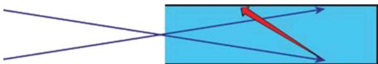
Figure 2.217 Cross-section of a Faraday cup for isotope ratio measurement, the large depth of the graphite cup prevents from losses caused by scattering. Arrows represent
